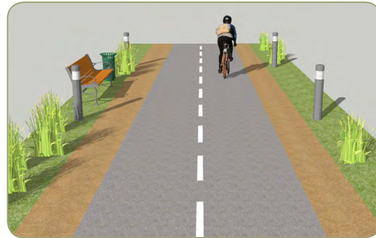
Figure 1.4: A Typical class I bikeway (Multi-use Path)
