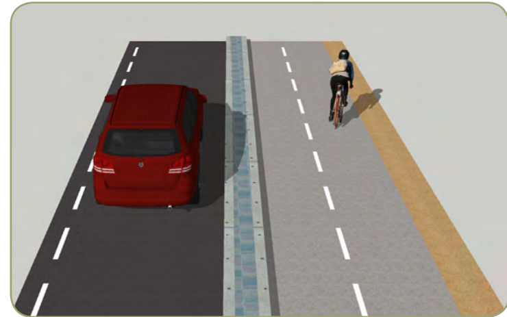
Figure 1.8: A typical class IV bikeway (cycle track)
