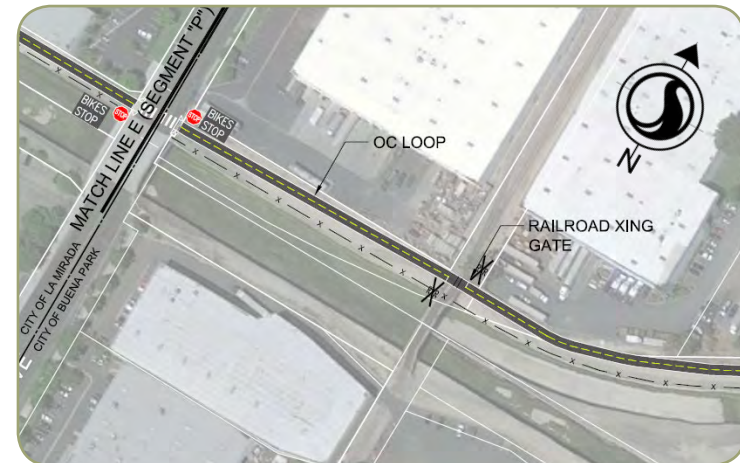
Figure 3.28: Proposed at-grade crossing of lightly used BNSF commercial rail spur, past Knott Avenue
