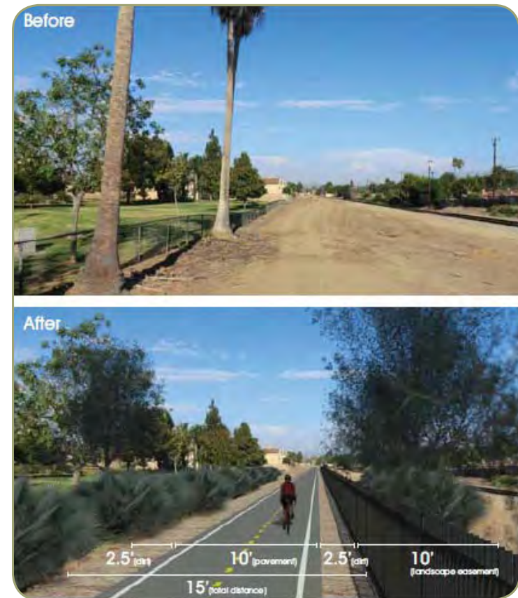
Figure 4.19: Before and After of proposed bikeway along UPROW (Source: 2013 UPROW Trail Feasibility Study)
