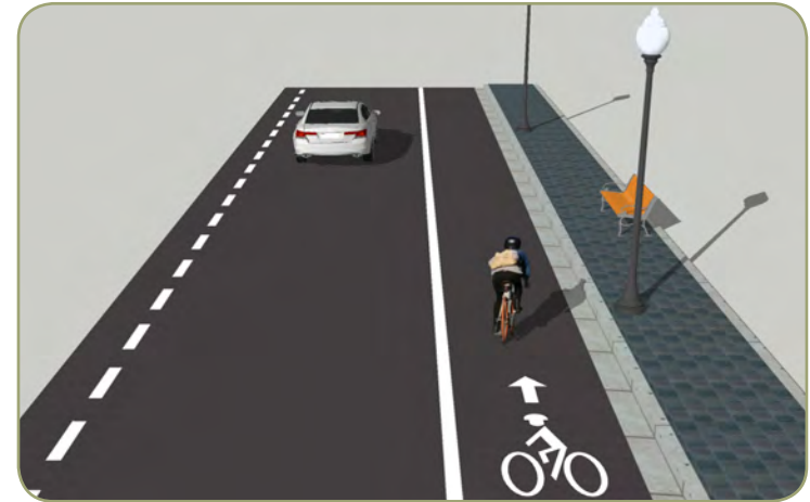
Figure 1.6: A typical class II bikeway (bike lane)
