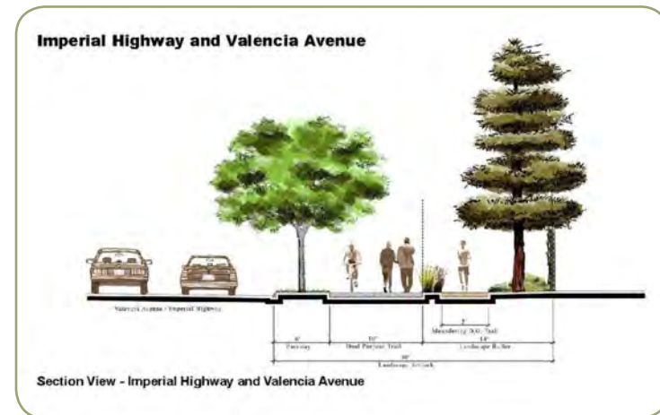
Figure 6.8: Cross section of a Bikeway along Imperial Highway (image from: City of Brea, Land Concern)
