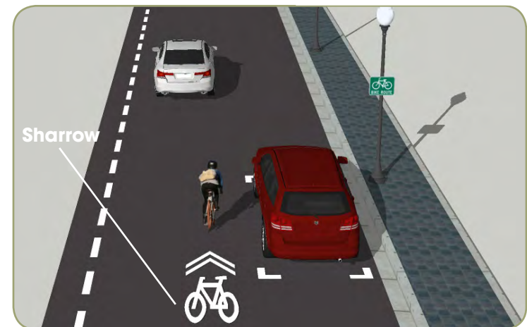
Figure 1.7: A typical class III bicycle route with sharrows
